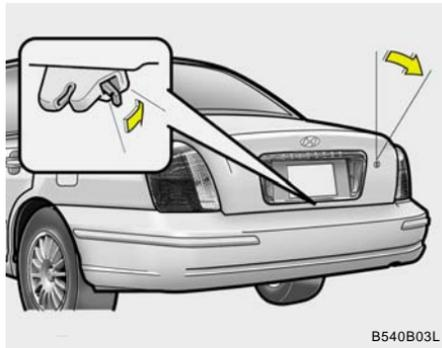
If the trunk lid lock knob (located near the latch) is in the "LOCK" position when the trunk lid is closed, it will not be possible to open the trunk lid by using the remote release. In this instance, use the master key to unlock and open the trunk lid.
