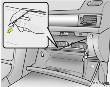
1. Open the glove box and take out the damper strap from the hole.
