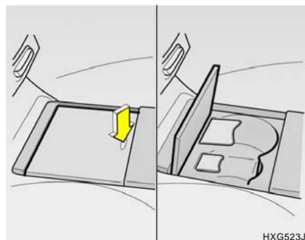
The drink holder is located on the main console for holding cups or cans. The drink holder can be opened by pushing at its top edge.
