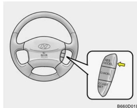
The vehicle will automatically resume the speed set prior to cancellation when you push the control switch "RESUME (ACCEL)" (above 25 mph).
