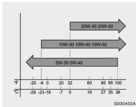
SH, SG or SG/CD (API) multi-grade and fuel efficient oil is recommended.
