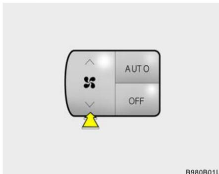
The fan speed can be set to the desired speed by pressing the appropriate fan speed control button. To increase fan speed press the  $\wedge$  arrow. To decrease fan speed, press the  $\vee$  arrow. The higher the fan speed is, the more air is delivered. Pressing the "OFF" button turns off the fan.
