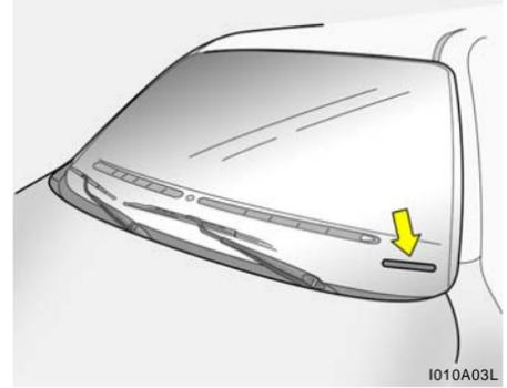
2. On the left top side of the instrument panel where it can be seen by looking down through the windshield.
