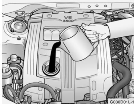
If the oil level is close to or below the "LOW" mark, add oil until it reaches the "FULL" mark.
