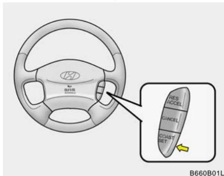
1. Push in the cruise control main switch. This turns the system on.
