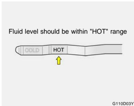
4. If the transaxle fluid level is low, use a funnel to add transaxle fluid through the dipstick tube until the level reaches the "HOT" range. Do not overfill.
