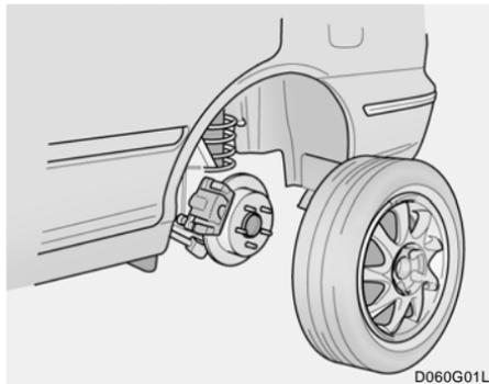
Loosen the wheel nuts and remove them with your fingers. Slide the wheel off the studs and lay it flat so it cannot roll away. To put the spare wheel on the hub, pick up the spare tire, line up the holes with the studs and slide the wheel onto them. If this is difficult, tip the wheel slightly and get the top hole in the wheel lined up with the top stud. Then jiggle the wheel back and forth until the wheel can be slid over the other studs.
