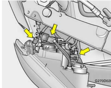
2. Disconnect the power cord from the bulb base in the back of the headlight.
