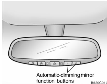
To assist you during nighttime driving, your mirror will automatically dim upon detecting glare from the vehicles behind you.
