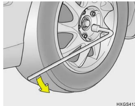
The wheel nuts should be loosened slightly before raising the car. To loosen the nuts, turn the wrench handle counterclockwise. When doing this, be sure that the socket is seated completely over the nut so it cannot slip off. For maximum leverage, position the wrench so the handle is to the right as shown in the drawing. Then, while holding the wrench near the end of the handle, pull up on it with steady pressure. Do not remove the nuts at this time. Just loosen them about one-half turn.
