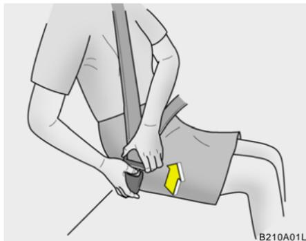
The seat belt is released by pressing the release button in the locking buckle. When it is released, the belt should automatically draw back into the retractor. If this does not happen, check the belt to be sure it is not twisted, then try again.
