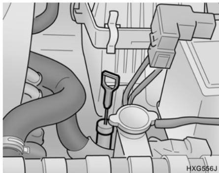
While the engine is idling, apply the brakes and move the gear selector lever from "P" to each of its other positions -- "R", "N", "D" -- and then to "N" with the engine still idling:
