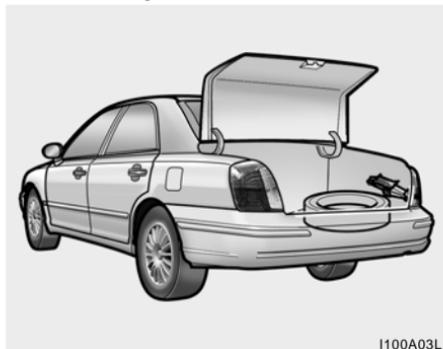
Remove the spare tire and take out the jack and tool bag from the trunk.
