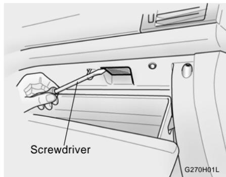
2. Remove the glove box illuminated light cover with a blade screwdriver.
