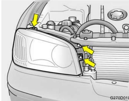
4. Using a socket wrench of the correct size, remove the headlight assembly mounting bolts.
