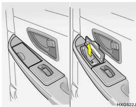
The rear ashtray may be opened by pulling the ashtray lid out. To remove the ashtray to empty or clean it, lift the metal ash receptacle upward and pull it out.
