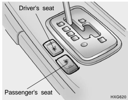
The seat warmer is provided to warm the front seats during cold weather. With the ignition key in the "ON" position, push either of the switches to warm the driver's seat or the passenger's seat.
