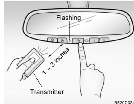
2. Hold the transmitter of the device you want to program 1 to 3 inches away from the bottom of the mirror. Simultaneously press the handheld transmitter button and the HomeLink button you wish to program. The indicator light will flash slowly at first, then rapidly, indicating successful programming.
