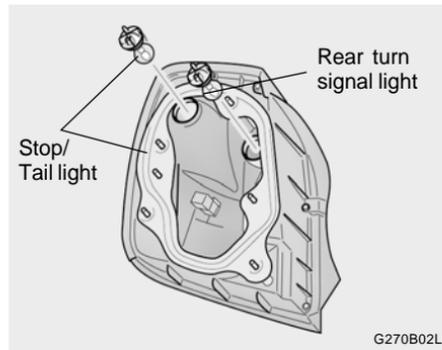
3. To replace the rear combination light (stop/tail light and rear turn signal light), remove it from the bulb holder and install the new bulb.
