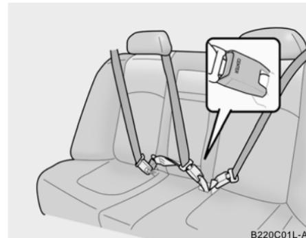
When you want to release the seat belt, press the button in the locking buckle.
