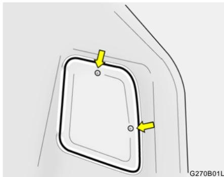
2. Remove the cover on the inside of rear luggage trim by unscrewing the screws.
