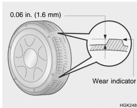
The original tires on your car have tread wear indicators. The tread wear indicators appear when the tread depth is 0.06 in. (1.6 mm). The tire should be replaced when these appear as a solid bar across two or more grooves of the tread. Always replace your tires with those of the recommended size. If you change wheels, the new wheel's rim width and offset must meet Hyundai specification.
