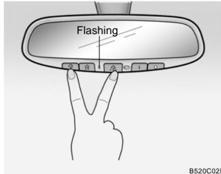
1. When programming the buttons for the first time, press and hold the two outside HomeLink buttons (⏏, ⏏), releasing when the indicator light begins to flash (approximately 20 seconds). This procedure erases the factory-set default codes. Do not perform this step when programming additional transmitters.
