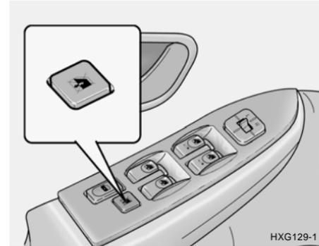
In order to prevent operation of the passenger front and rear windows, a window lock switch(2) is provided on the armrest of the driver's door. To disable the power windows, press the window lock switch. To return to normal operation, press the window lock switch a second time.
